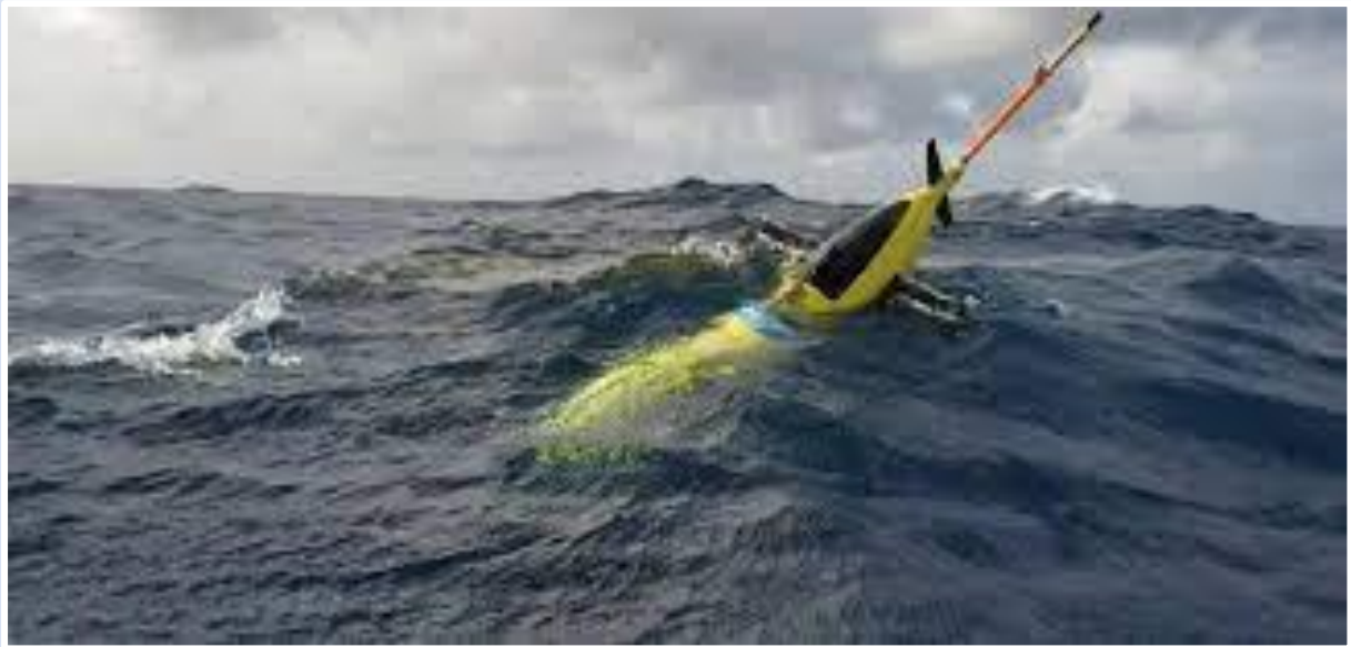
NOAA underwater glider, an autonomous underwater vehicle (AUV) being launched
