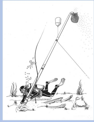
Illustration of a dive sand lifter in operation
